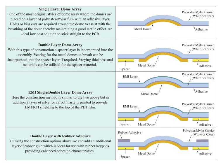
Dome Arrays can be manufactured as simply as say one or two domes on a polyester backing to large panels which may incorporate a large number of domes in a pattern to suit a custom application. Different size/types of domes can be incorporated into the array design.
